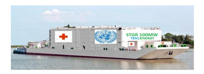
MPB RDR: 40 MW POWER BARGE Length: 145 m. - Width 36 m. - DAMEN Shipyards.SMR Small Modular Reactor:  $2 \times 20 \text{ MW STGR STATIONS } L \times W \times H = 15 \text{ m.} \times 10 \text{ m.} \times 14 \text{ m.}$ MED: Multi Effect Distillation  $-4 \text{ units } 2500 \text{ m}^3/\text{day} - L \times W \times H = 15 \text{ m.} \times 5 \text{ m.} \times 12 \text{ m.}$
